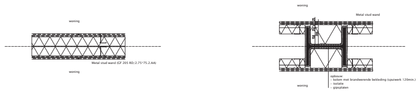
▲ VENHOEVENS ARCHITECTURE+URBANISM – DETAILS (PARTITION) WALL
